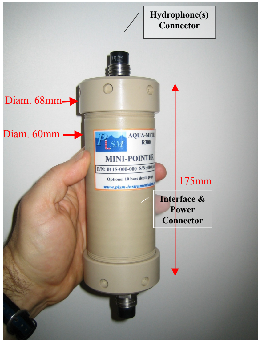
Mini-Pointeur R300 (hydrophone not plugged)
