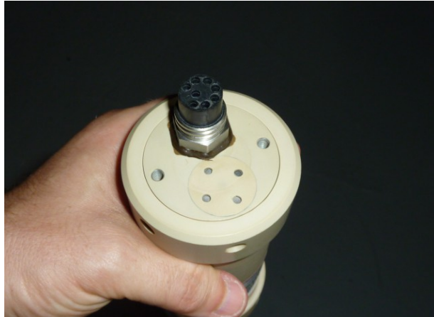
Bottom Interface & Power Supply Connector
