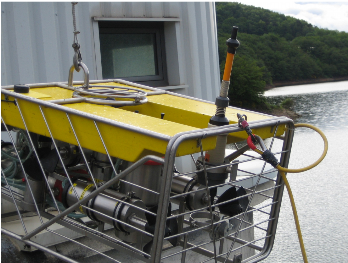
MiniPointer installed on a light survey class ROV
