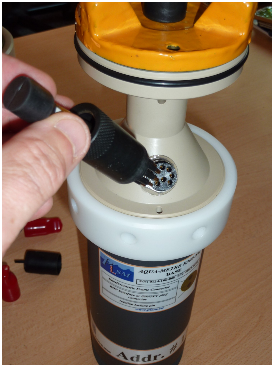
Plugging On/Off dummy plug (for remote acoustic mode)
